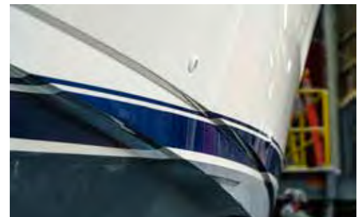
Exterior Trim is responsible for enclosed bridge installations and application of boot and accent stripes.
