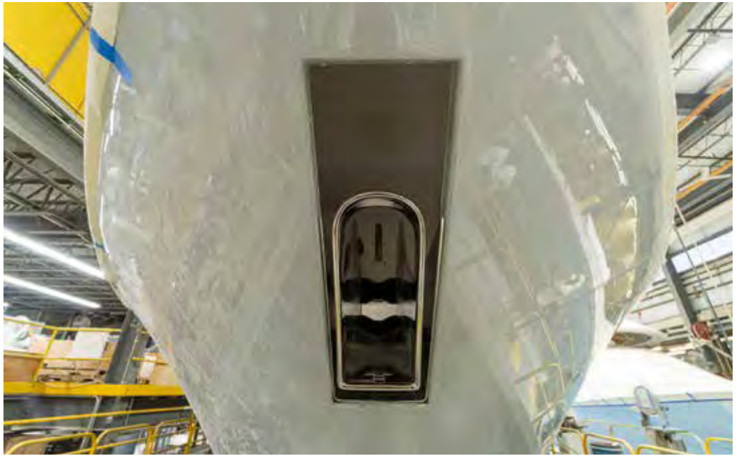
It takes a team of shipwrights from Exterior Trim to insert the stainless steel through-stem anchoring system in a Viking 92.
