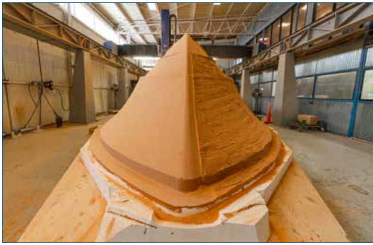
Our 5-axis CNC router makes the final cut to the hull plug (consisting of a cured epoxy covering a foam structure).
