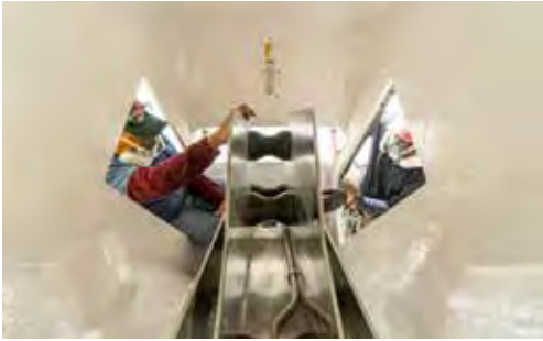
It takes a team of shipwrights from Exterior Trim to insert the stainless steel through-stem anchoring system in a Viking 92.
