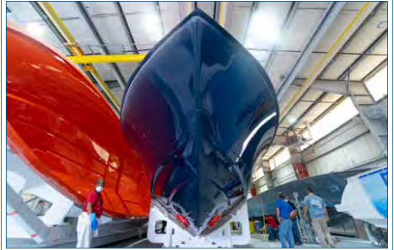
Hull No. 1 is pulled from its mold, which is held in a custom hydraulic turning rig.
