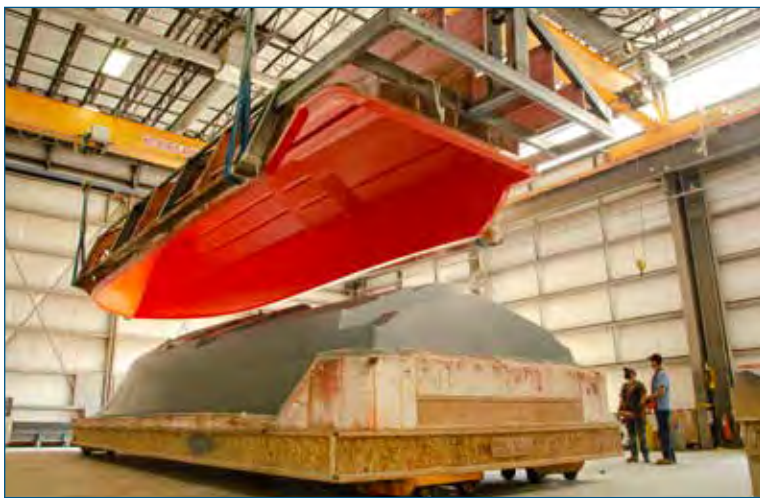
The hull mold, which will be used to build the boat, is lifted from the finished plug.
