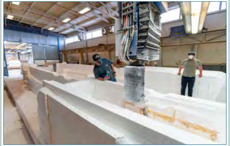
The rough cut of the structural stringer grid's foam plug.
