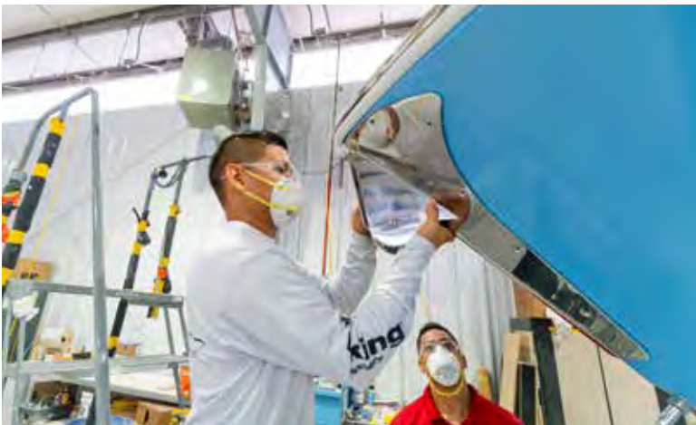
Viking Mullica has its own Trim Department. Antonio Laines gets the stainless steel bow roller in place on a V-33, followed by its anchor windlass.
