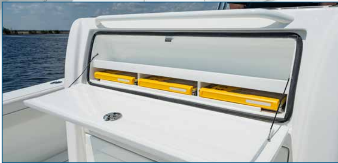
The helm seating module features a custom Valhalla cooler with seating pad, a drawer and a tackle locker with door that doubles as a rigging table when open.
