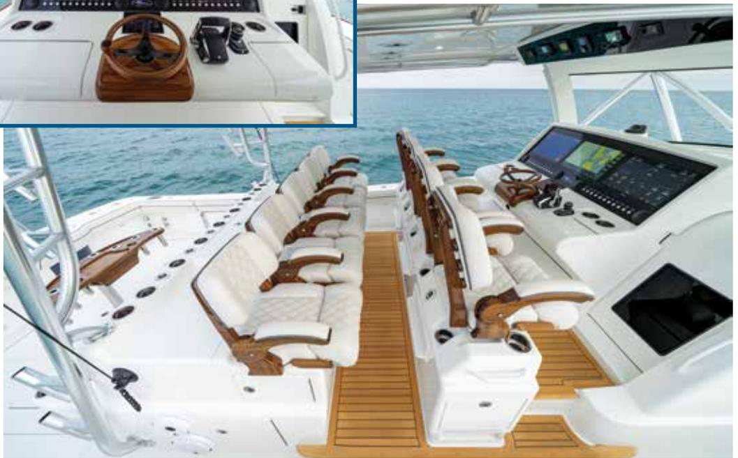
Port and starboard glove boxes house a variety of instruments and controls, including the fuel tank selector switches, Hooker live well variable speed control knobs and bow thruster control. Above, you have a molded-in pod in the hardtop for VHF radios and monitors and controls for various systems, such as the Seakeeper, water maker and a Garmin marine instrument display.
