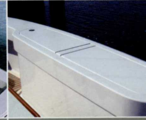
Transom Fishwell: The molded fishwell features locking latches and overboard drainage.
