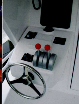
Upper Control: Aft bridge station for docking and fishing.
