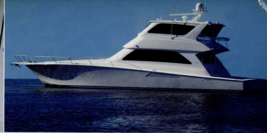
Style and Substance: For strength and durability, the enclosed bridge is a one-piece unit that becomes integrated into the yacht.
