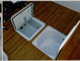
Fish House: Insulated fish, live bait and stowage wells are deeply guttered to drain run-off water. Hatch bottoms are finished smooth for easy clean up.
