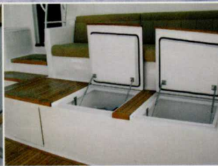
Deep Freeze: Under-mounted freezers mean more capacity for bait and food. Engine room access is to port.
